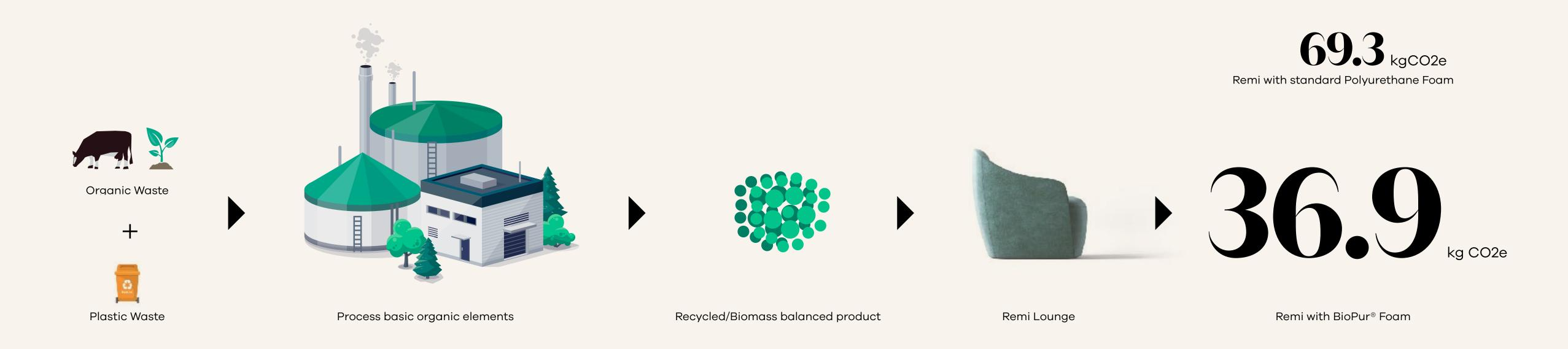
BioPur® Foam is an innovative type of polyurethane foam that incorporates bio-based materials as a significant component of its formulation. This eco-friendly alternative to conventional foam is designed to offer similar, if not superior, performance characteristics while substantially reducing environmental impact.
